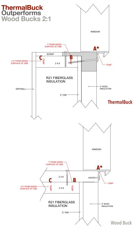
\* ThermalBuck reduces heat transfer vs. wood 54% at Point A.
